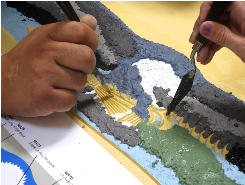
Figure 2 — Craftsmen use artists' palette knives to place and consolidate polychrome mosaic concrete mixtures into molds with ridges outlining every small area of color in the artwork.
